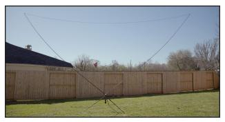
3. Fully extend both whips to finish deployment.
